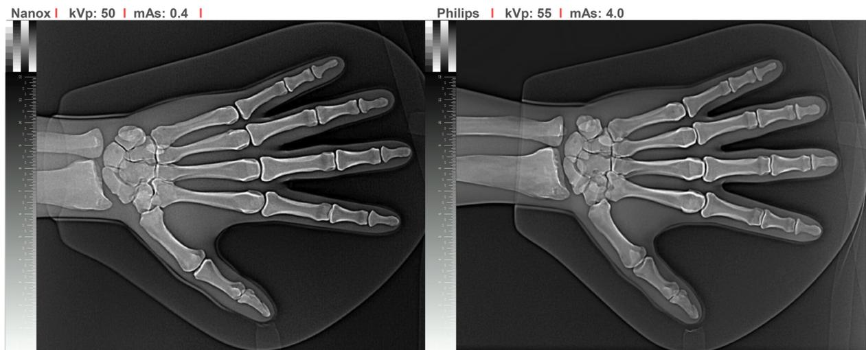
**kVp** - Kilovolt Peak. kVp is the component that controls the X-Ray penetration strength and subsequently **QUALITY** of the X-Ray beam produced. It is also what controls the **CONTRAST** or **GRAY SCALE** in the produced X-Ray film. The Higher the **KVP** the **LOWER** the **CONTRAST**.
