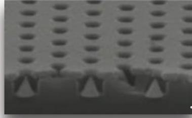
**100 Million nano-cones** field on a silicon chip emitting digitally controlled electron streams under low voltage
